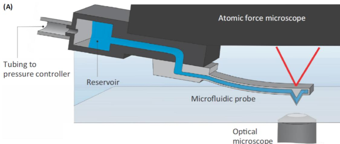
**Figure 1.** Principle of FluidFM technology. Reprinted from <sup>1</sup>.
